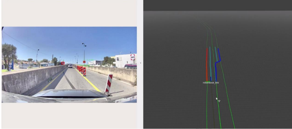
Figure 18 The environment and data gather (left). The lane boundary (red) based on HD Map(green) and Final system shows the updated HD-map
