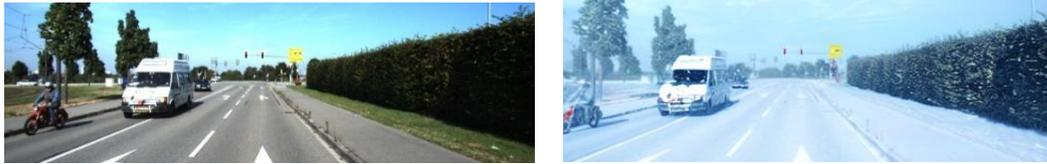
Figure 1: Original image (left), synthesized via pix2pix (right).
