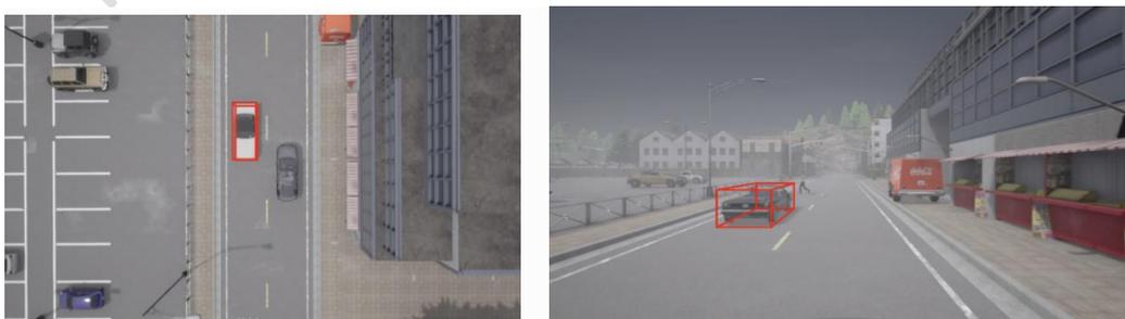
Figure 9: Oncoming car ground truth bounding box display during runtime (snapshot from Scenic-CARLA co-simulation environment)
