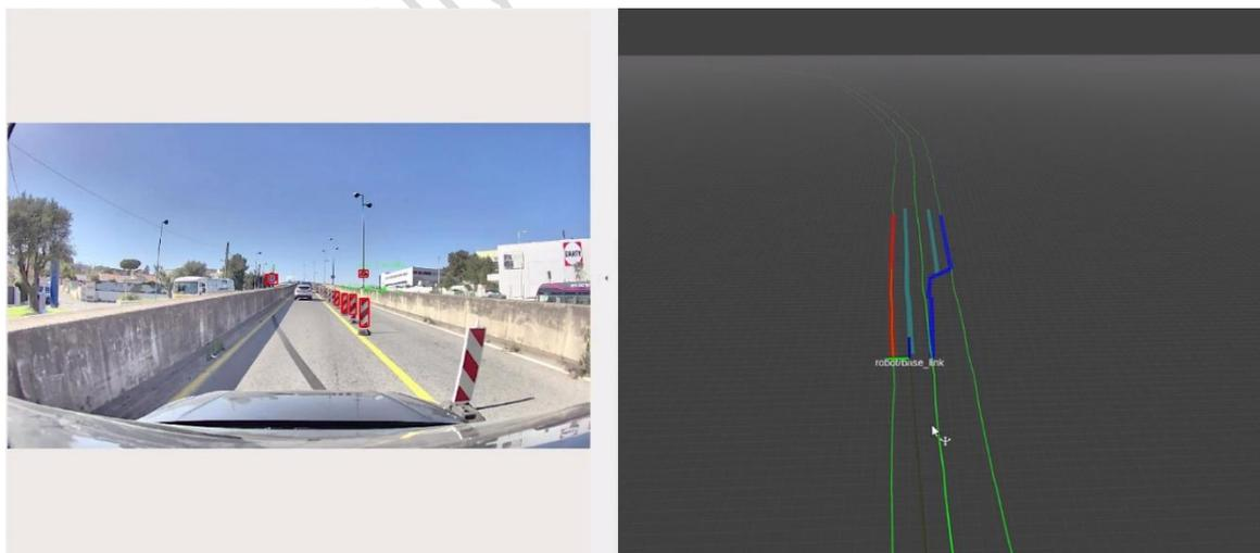
Figure 42: Final system shows the updated the HD-map. Example is shown in the map frame (against the original map frame HD-map shown by the green lines). The red lines on the right panel are the left boundary of the drivable road, and the blue line is the right boundary of the drivable road. The light blue lines are the centerlines of the lane/s.
